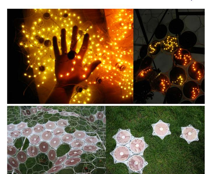
A modular photovoltaic membrane was prototyped for the installation that can be clad to synthetic textile architecture to provide both shelter and shade from the sun during the day and once evening falls light is cast into the darkness using low-power micro LEDs with printed circuitry. Loop.pH will be developing this over the next 12 months as a low cost, high volume source of light for emergency shelter relief – in places where light and electricity are not provided.
