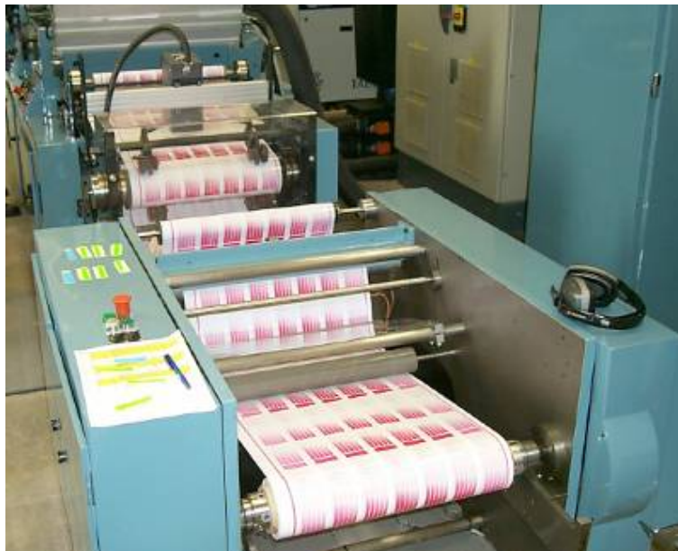
Printing presses enable roll-to-roll production at a rate of 80m/minute on a 600mm web
