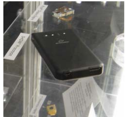
The Microvision SHOW pico projector prototype uses a single bi-axial scanning mirror assembly. This is a MEMS device, and the mirror is only one millimeter in diameter.
