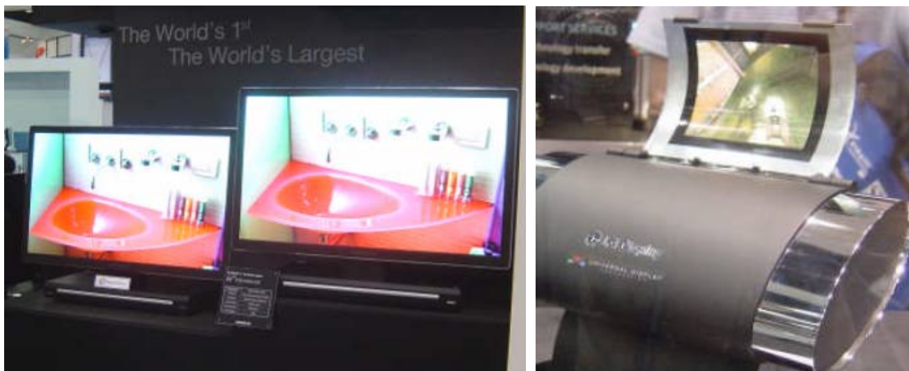
On the left are samples of Samsung's 31-inch AMOLED display. On the right is a prototype from LG Display using Universal Display's OLED materials demonstrating the flexibility of the technology.
