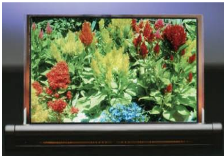
4.3-inch diagonal full colour OLED display made with DuPont materials and Dai Nippon equipment.
