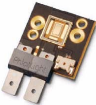
The Luminus Devices PhlatLight LED chip used in RPTV applications is pictured on the left. On the right is a prototype desktop panorama display using Osram LED illumination. The system is expected to be available Q4'08.
