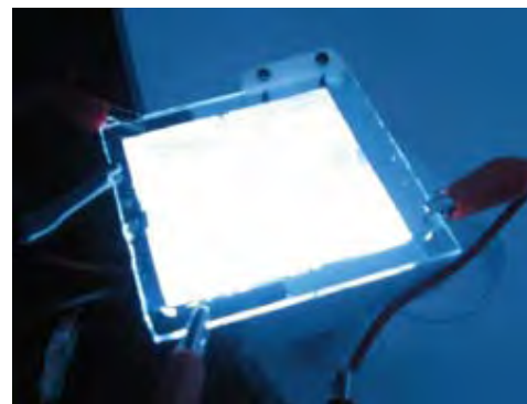
Achievements after the first year of Project Topless include a two-fold increase in efficiency and life, >7 lm/W -1 at 500 cd/m -2 life at about 21Khrs, a single white light emitting polymer in a single pixel device (25cm 2 ), showing good brightness and colour uniformity.
