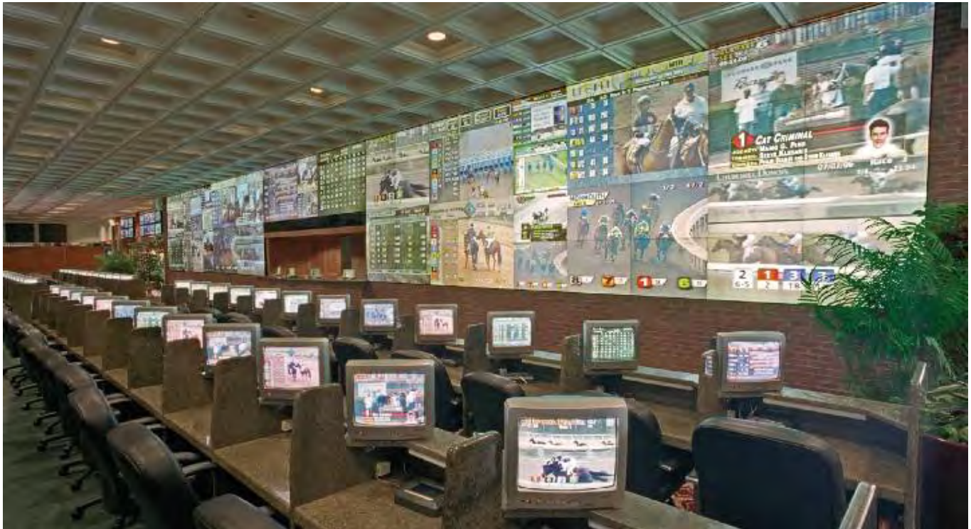
82 "cube" videowall, based on 50-inch modules, at Delaware Park Racecourse – 63m 2 display area
