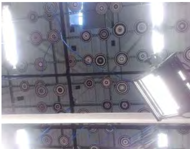
The scale of DMU's facility is impressive – this is for 3D tracking, with numerous camera views and ceiling markers
