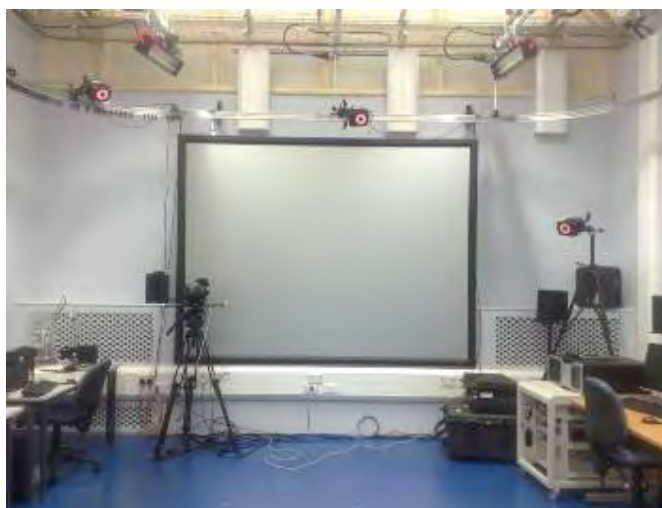
The scale of DMU's facility is impressive – this is for 3D tracking, with numerous camera views and ceiling markers
