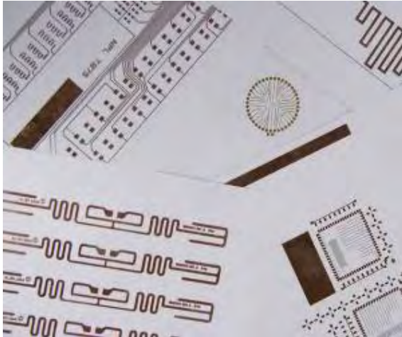
CIT prefers to use copper on PET, but can work with a variety of metals on numerous different substrates
