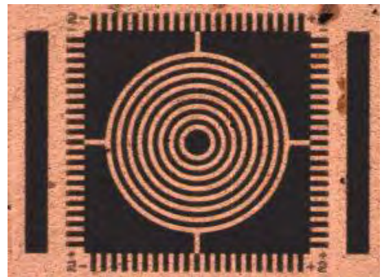
The CIT process can enable very fine line structures, as small as 2.5 microns, which is invisible to the naked eye
