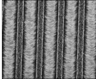
Graphic illustrates a single row of nanowires (cylinders with red tops) with fin-shaped nanowalls extending outward; the transmission electron microscope image shows four rows of nanowires and their corresponding nanowalls. They are called “nanoLEDs” because they emit light when electrically charged. The distance across the micrograph is approximately the diameter of a human hair; Transmission electron microscope image of “nanoLEDs” emitting light
