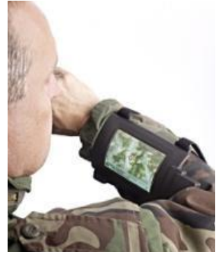
A wrist mounted flexible OLED display and communications device built on thin metal foil, which uses Universal Display's highly efficient phosphorescent OLED technology and materials.
