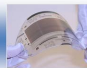
Debonded substrate Mechanical Release No TFT degradation No residue No carrier damage
