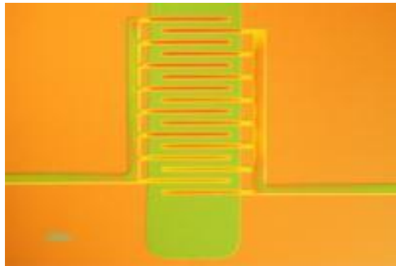
Princeton researchers have developed a plastic process for ink-jet printing conductive polymers shown here in a plastic transistor with interdigitated source and drain (orange) allowing current flow down the active channel (green).
