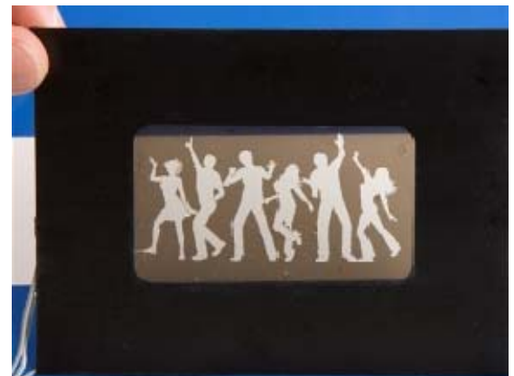
HP Electronic Skins, or eSkins, is a flexible reflective color film that can be applied to a variety of consumer electronic devices for product personalization
