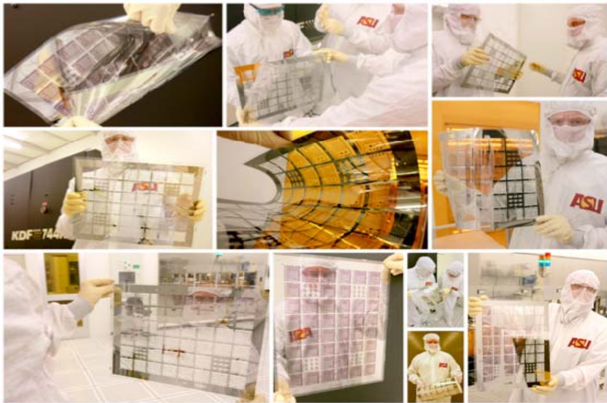
Amorphous Si TFTs on Temporary Bonded GEN II HS-PEN in Process at the Flexible Display Center
